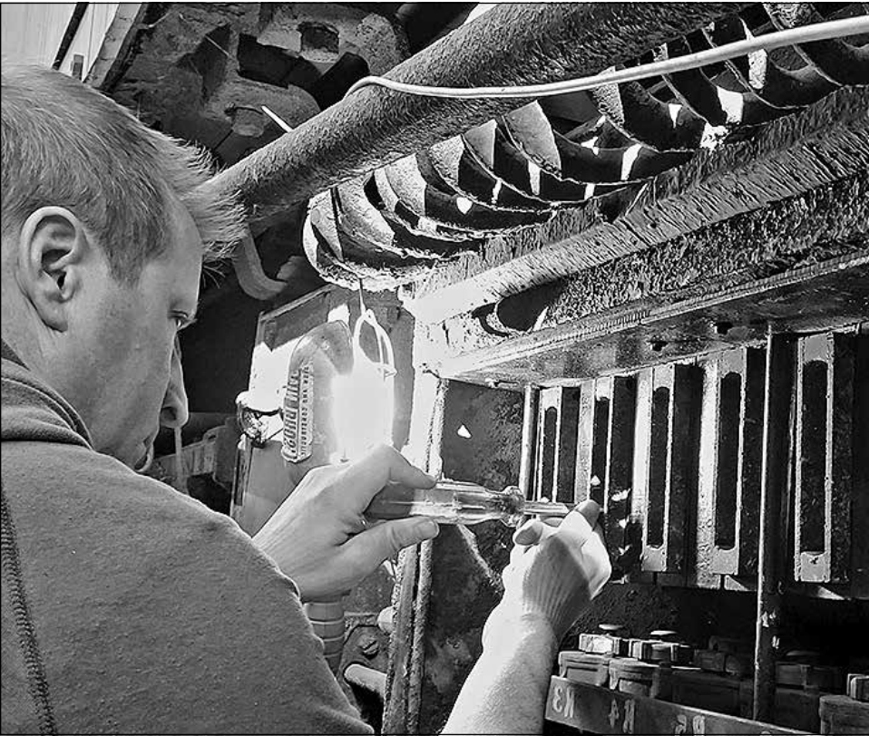
Eric Zabelny works on cleaning and replacing the interlocks and relays on Car 228.
