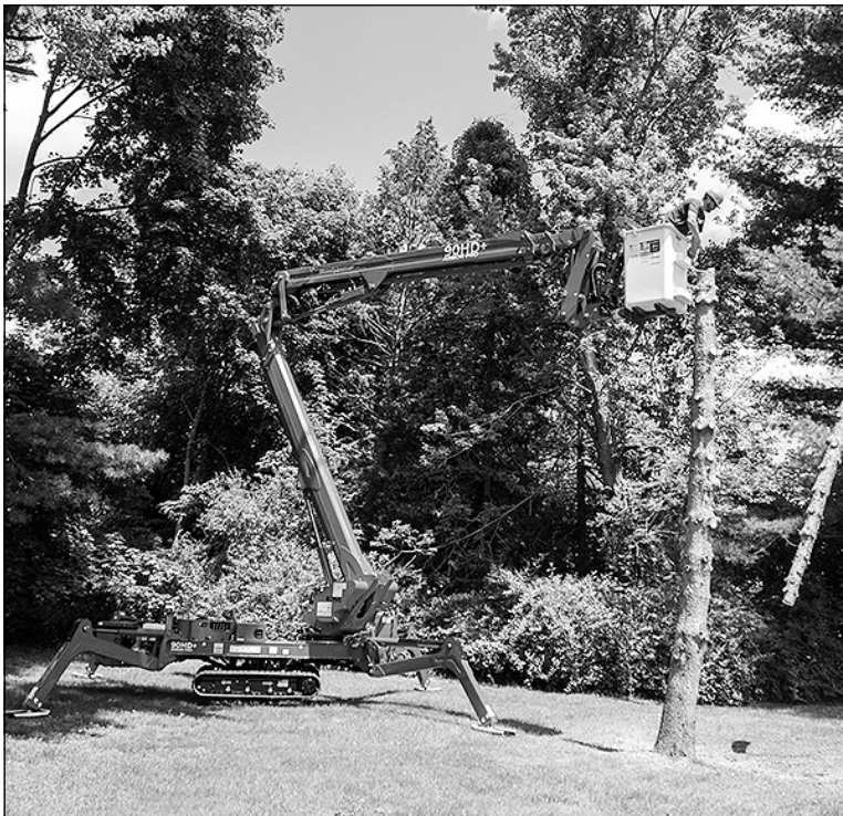
This spider lift is one of the many pieces of equipment that Double K uses in its work.
